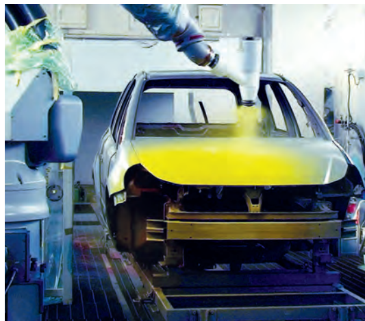
The top coat is applied to an automobile body at a Kansai Paint painting booth at a factory in Japan.
